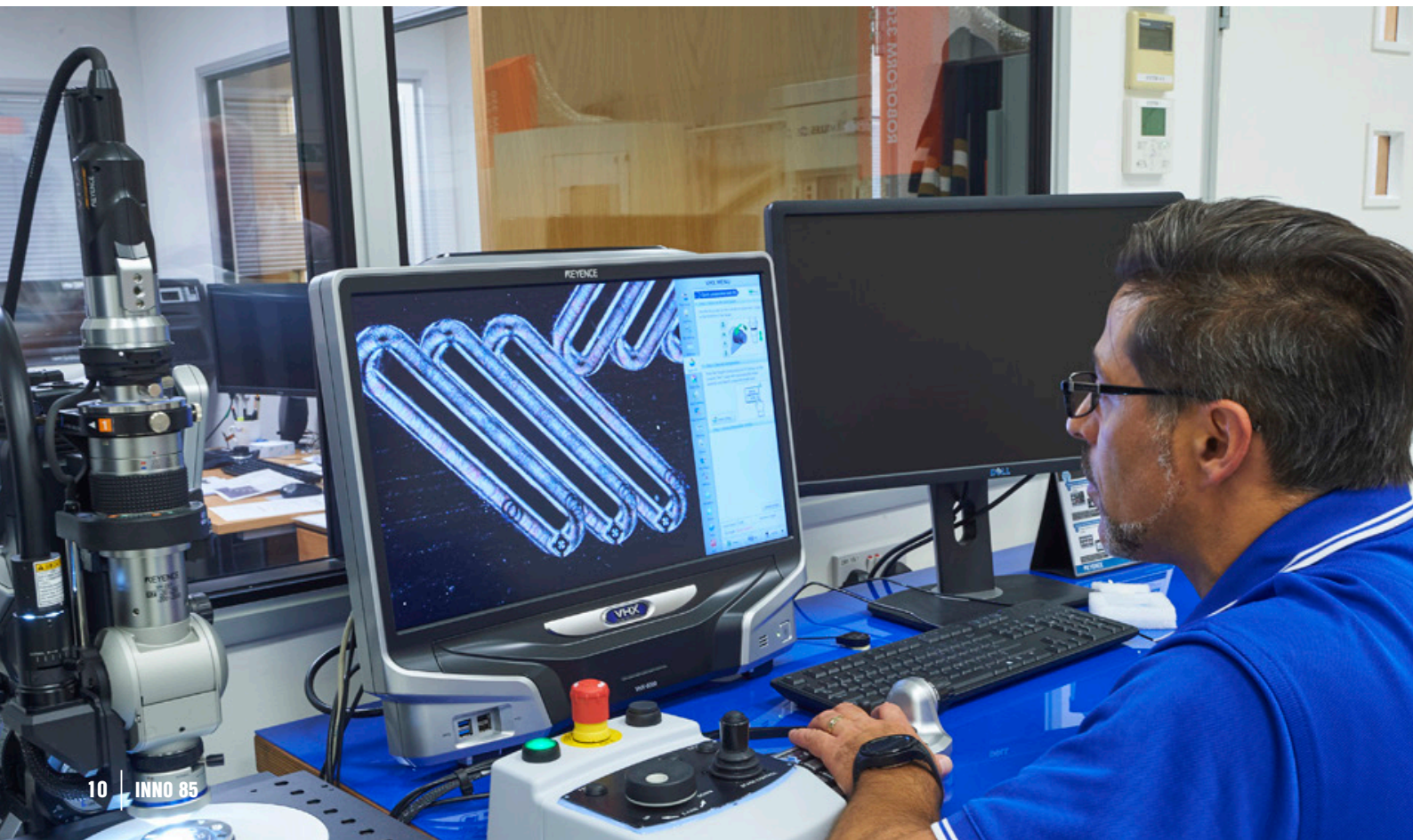
Figure 1: Microfluidic chips with incorporated 30-micron microchannels, integrated optics features and a surface finish of less than 20-micron Ra.
